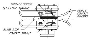
A copper alloy housing supports the reverse loop, silver plated copper female contacts. These female contacts are backed by insulated stainless steel compression springs which apply pressure to the blade providing low resistance current transfer. As the blade enters, it forces the contacts apart, thus providing a wiping and self-cleaning action of the contacts.
